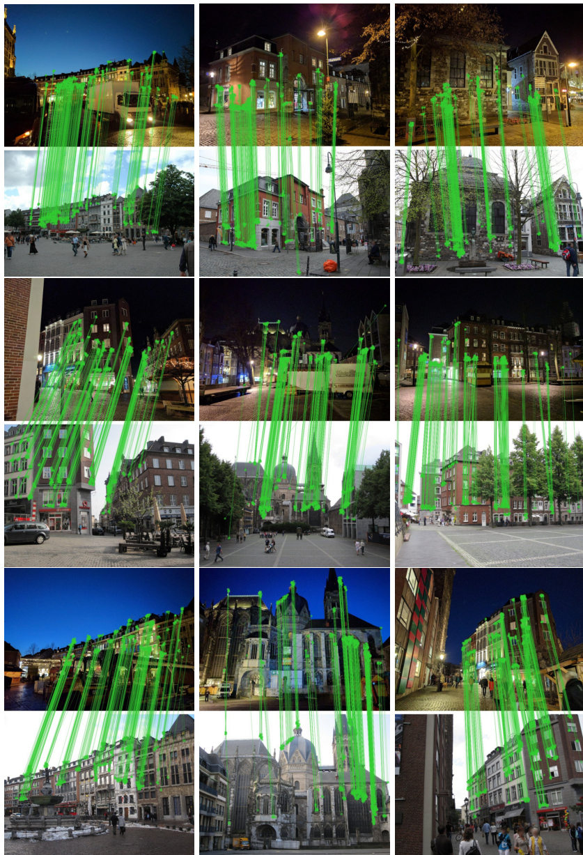
Fig. 11: Aachen day-night results. We show the top 500 correspondences obtained by Sparse-NCNet between the night query image (top) and the database day image (bottom). Note that the large majority of matches are correct, despite the strong illumination changes.
