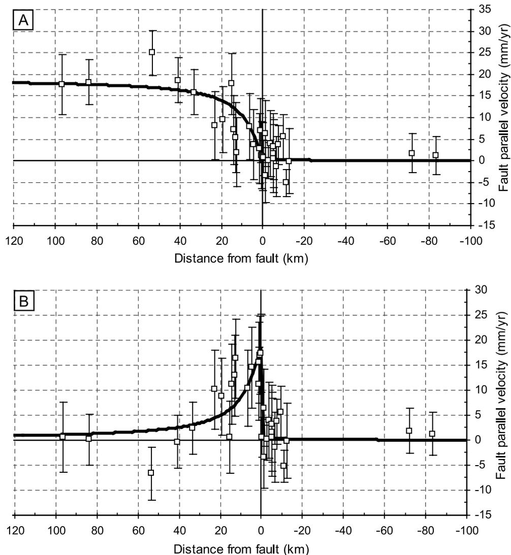
**Figure 3.** (a) Observed and (preferred) modeled fault parallel motions along the Sumatra Fault near lake Toba caldera. Observations are from *Genrich et al.* [2000] relative to stable Sunda/Eurasia plate for the Sidikalang and Dolok Sanguul transects. (b) Same as in Figure 3a but only showing the effect of elastic loading itself along the main fault. Uncertainties in observed velocities represent one standard uncertainty.
